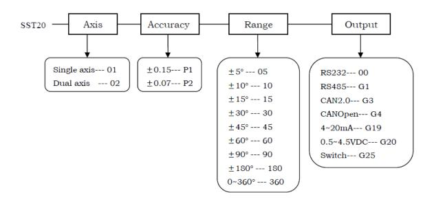
**Remarks:** 4~20mA and 0.5~4.5VDC output inclinometer only provide 0.15°accuracy class; RS232/485, CAN2.0, CANOpen and switch output inclinometer only provide 0.07 accuracy class.
